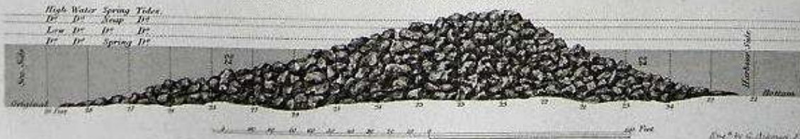
TRANSVERSE SECTION of the FINISHED PART of the BREAKWATER.
