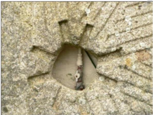
Millstone 6: detail of eye and rynd chases
