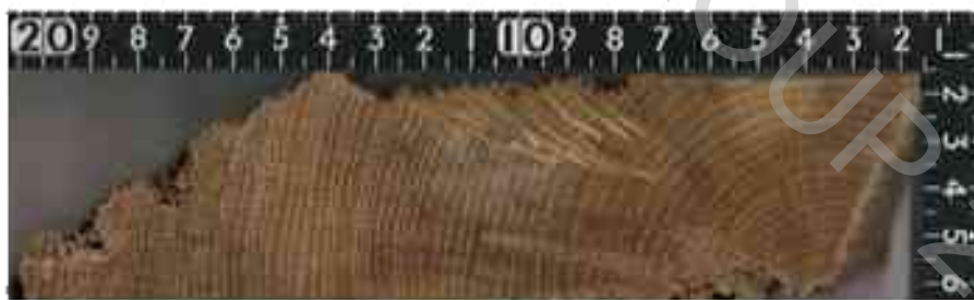
Photo 6: Section of oak from Joist 4 (series INM102)
