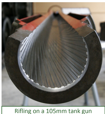
Rifling on a 105mm tank gun
